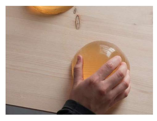
The ballistic gel is a gel that mimics the human body mass. It is used as a substitute for the body to simulate for instance bullet impacts.
